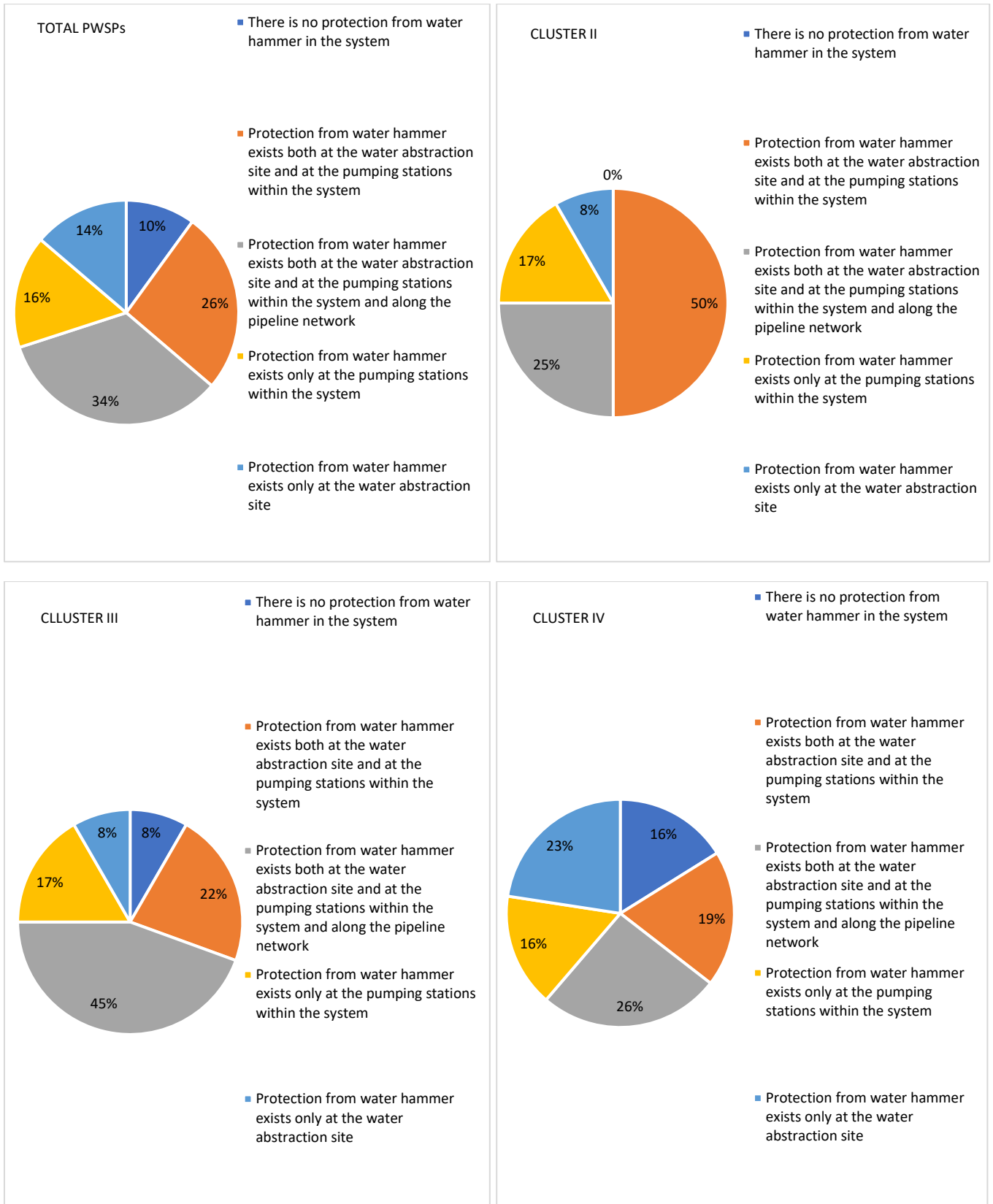
Figure 2.24. How water hammer protection is implemented on the national level and by PWSP clusters
