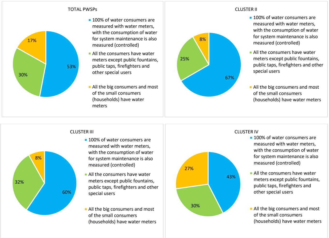
Figure 2.95. Way in which consumption by users is measured by individual PWSPs on the national level and by clusters 36
